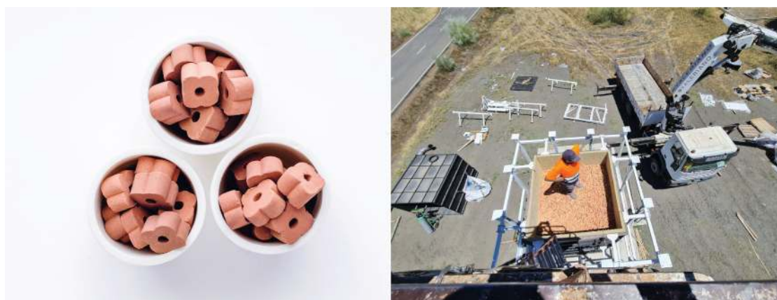
Fig 1: Pictures of (a) ReThink Ceramic Flora, the world's first 100% recycled material for high temperature thermal energy storage applications commercialized by Seramic Materials Ltd., and (b) 25 tons of Flora tested in StorEnergy's pilot located in Plataforma Solar de Almeria (PSA) in Spain
