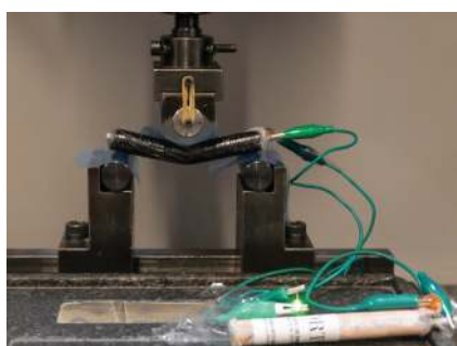
Figure 1: Beam-type structural battery loaded in three-point bending.
